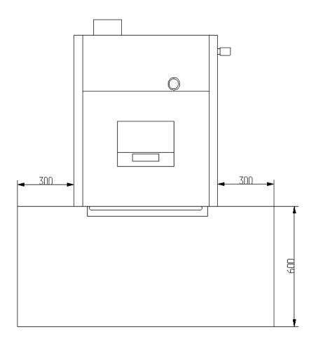
Recommended clearances for BM 25,40,60,80 (in mm)
