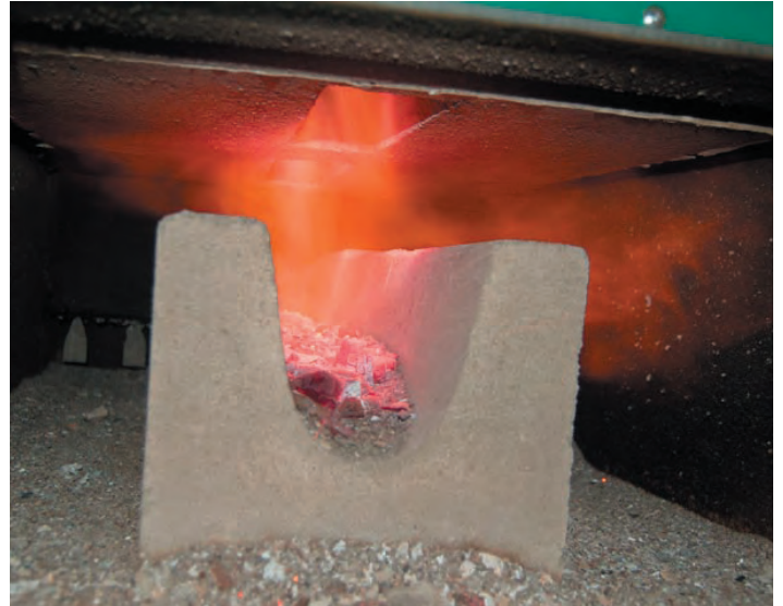
Two views of the gasification chamber and nozzle burning at near 2,000 degrees, F.
