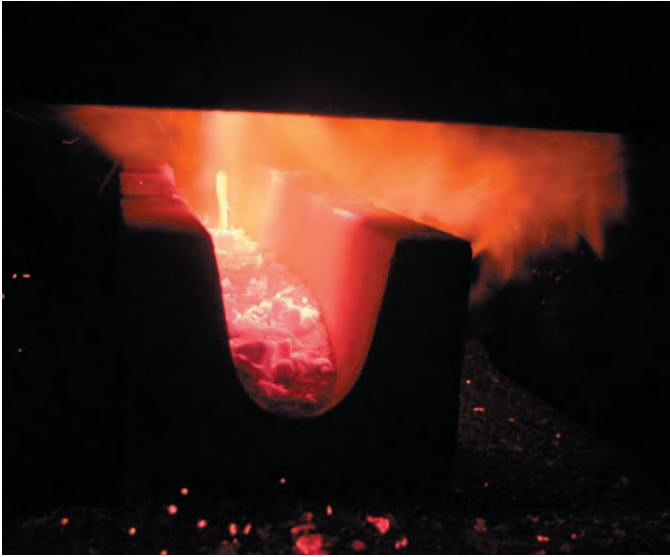
Two views of the gasification chamber and nozzle burning at near 2,000 degrees, F.
