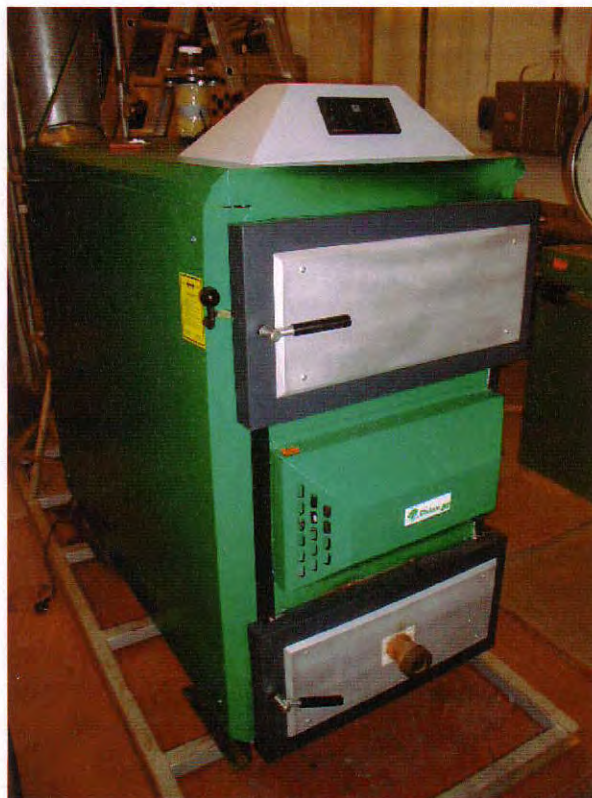
Fig. 5: - overall view of the boiler (with a combustion chamber test door and covered fan)
