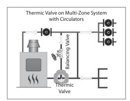
Where a high mass non-condensing heat source is matched with a large low temperature system, a situation could occur where the heat source is unable to maintain the rate of demand from the system. The use of the thermic valve provides the opportunity for the heat source to catch-up.
