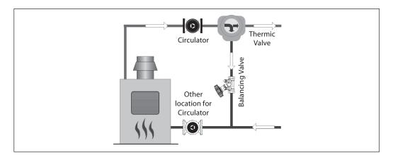
Gravity conversion systems contain an enormous volume of water, and the water returning to the heat source could be significantly cooler, leading to condensation
