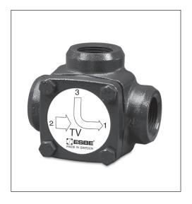
The ESBE thermic valve is a boiler by-pass valve that prevents cool return water temperatures in a hydronic heating system. The purpose is to safeguard conventional non-condensing boilers against corrosion from condensation that would result if a minimum flue gas temperature is not maintained.
