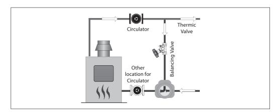
Where a high mass non-condensing heat source is matched with a large low temperature system, a situation could occur where the heat source is unable to maintain the rate of demand
