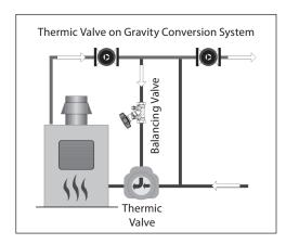
Gravity conversion systems contain an enormous volume of water, and the water returning to the heat source could be significantly cooler, leading to condensation and a shorter life for the heat source. Adding a thermic valve to the system will prevent the boiler from sustained operation at temperatures resulting in condensation.
